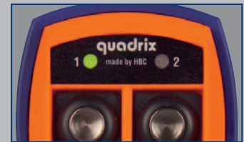
Indication of preselected trolley or hoist by 2 LEDs.
