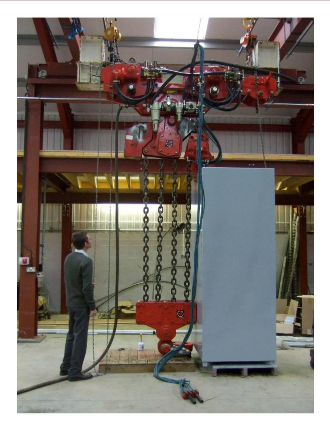
50 Tonne Hoist & Trolley with 50 metre Height of Lift With Special Design Heavy Duty Chain Collector
