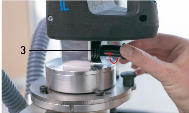
With the regulating screw for the transport goods (3) it is possible to regulate whether air-tight or porous materials are suctioned. If it is closed, it is possible to lift air-tight transport goods. To lift heavy cardboard boxes, the screw has to be unscrewed some, while to lift sacks or bags it has to be unscrewed completely.
