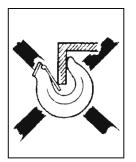
Fig 4 d Hook tip subject to additional bending stress!
