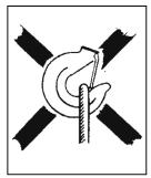
**Fig 4 a** The sling is applying load to the hook tip!
