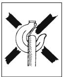
Fig 4 c Hook latch obstructed!
