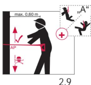
Work positioning according to EN 358 /
