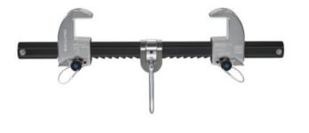
The BEAMTAC 2.0 mobile anchoring device is suitable for use as an attachment clamp for steel beams with a flange width of 90 to 380 millimetres and can be used for many different kinds of work in an industrial environment.
