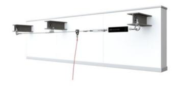
Traversable lifeline systems ABS-Lock SYS II (8 mm) & IV (6 mm) for overhead installation. Overhead-mounted lifeline systems greatly reduces the risk of a swing fall. Ideal for overhead usage or on a facade. The connector between the user and the fall arrest system is kept relatively short to reduce the fall distance and the risk of sustaining injury through hitting the ground.
